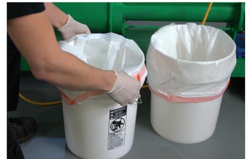
7) You will need two 5-gallon pails during operation. One pail for priming the Green Machine system on startup, and one pail for clean-up. Lining the pails with a trash bag will make disposal and reclaiming material easier.
