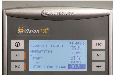
12) Change the cavity speed to 30% then press the enter key.
