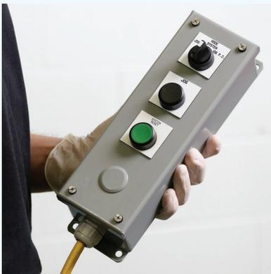
Use the remote to perform some basic functions without using the control panel, including starting and stopping.
