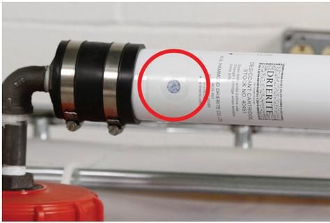
1) Check the inspection window on the desiccant holder. If the window is blue, proceed. If the window is pink, replace the cartridge.
