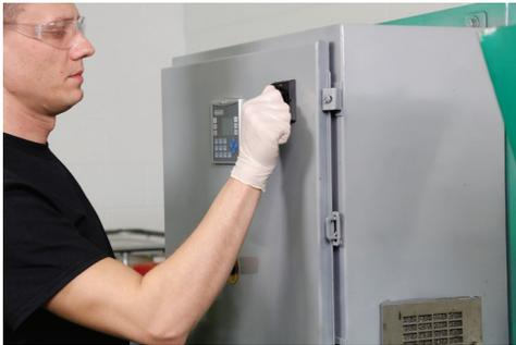
4) Turn the power switch on the control panel to the ON position.
