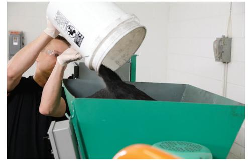
3) Check the level of the filler/grind in the hopper, add filler if needed.
