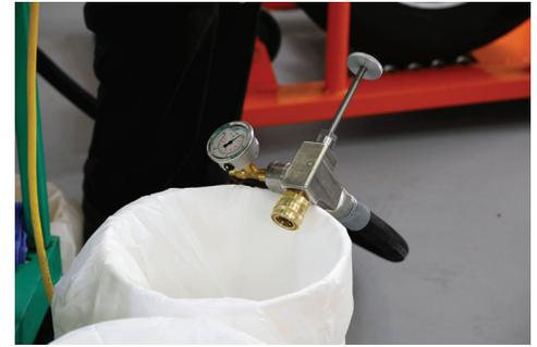
10) The Green Machine must be primed before tires can be filled. To prime the Green Machine, place the fluid gun over a waste container. Select jog P.C. on the remote and press the jog button until all the solvent has been removed from the mixing well.
