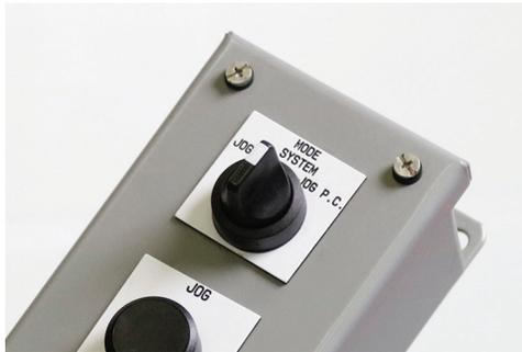
11) Change the remote to System and reduce the cavity speed to 30%. To adjust the progressive cavity pump speed, press the enter key on the main control panel. The cavity speed percentage number will be highlighted.
