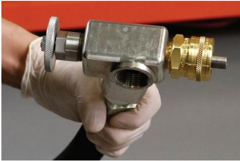
8) Remove the cap and connect the fluid gun body to the dispenser hose. If the fill gun plunger isn't already attached to the gun body, attach it now.
