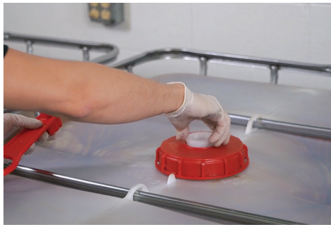
14) Open the white 2" bung to vent the CAT-side tote.
