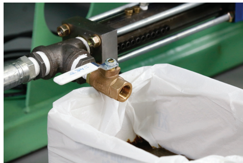
20) Place a disposable container under the sample valve assembly.
