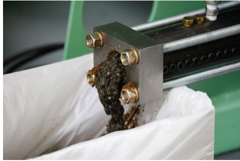
17) Jog the grinder for 15 seconds using the jog grinder forward button and run or jog the mixture through the injector until it flows freely. Ensure that both granulate and virgin TyrFil are extruding properly into a container. Then stop the AutoFil by pressing the stop button.
