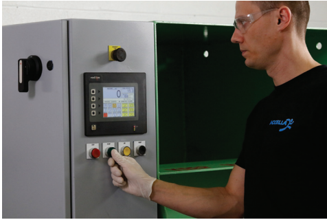
16) Turn the machine on and choose the 40/60 mix ratio.
