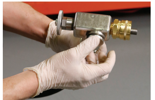
21) Connect the gun body to the other end of the hose. If the fill gun plunger isn't already attached to the gun body, attach it now.
