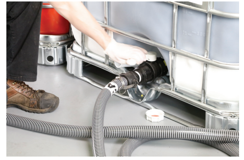
15) Open the ball valves on the ISO and CAT side totes.
