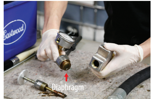
9) Remove the PSI gauge from the gun assembly. Clean the diaphragm thoroughly with a brush in 99% isopropyl alcohol. Store in a safe place.
