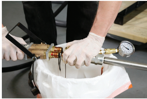
14) Disconnect the mixing tube from the manifold head, leaving the coupler on the head.
