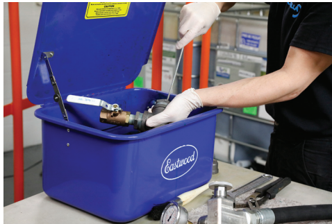
8) Thoroughly clean the sample valve with a brush and store in alcohol.
