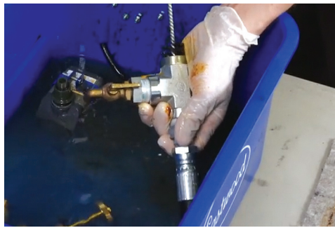
17) Lay the whip hose in solvent and clean the sample drain valve with a brush. Make sure the sample drain valve is open.
