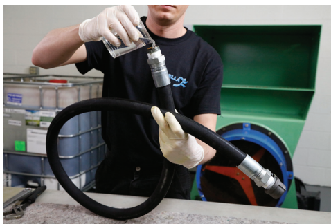
11) To clean the fill hose, put a cap on one end and fill with alcohol. Next put a cap on the other end of the hose.
