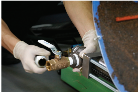
5) Remove the fill hose from the sample valve and allow it to drain into a suitable container.
