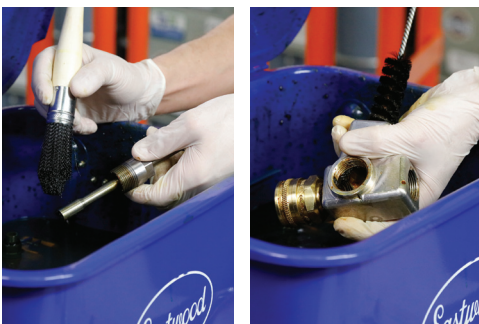
10) Clean the fill gun plunger and the gun body, rinse and store all parts in alcohol.
