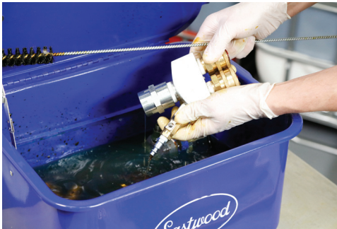
20) Open the manifold head pressure gauge valve and clean the manifold head connectors. Store the manifold head in the solvent.
