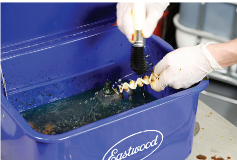
19) Clean the mixing elements in the solvent and store them in a safe place to avoid breakage.
