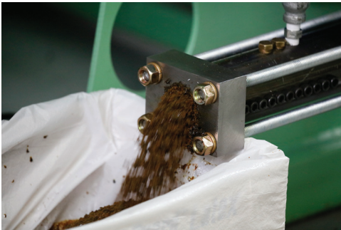
7) Next, release the emergency stop on the control panel. Run only the grind and injector until you have dry material exiting the barrel. Then press the emergency stop and turn the machine off at the main power source.
