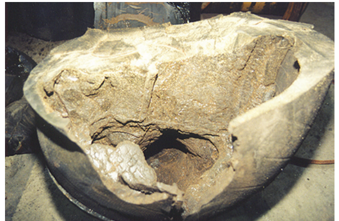
Photo IV: This picture shows what happens to a tire when the “Chunk” overheats. The “Chunked” core has disintegrated while the new virgin fill remained intact encapsulating the “Chunk”. The tire failed due to the failure of the chunk – it had approximately 2” of good tread life remaining when the carcass failed.
