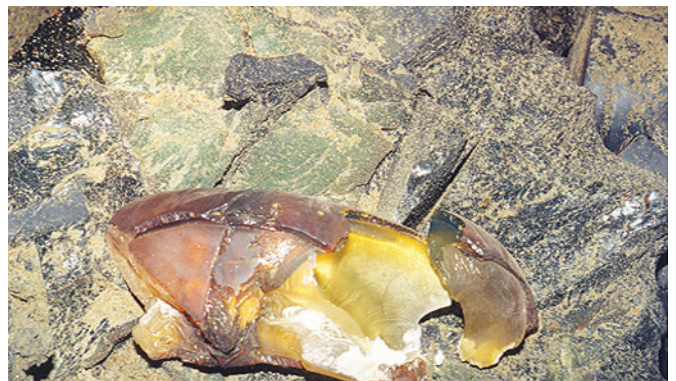
Photo I: This picture above shows 3 distinctly different (incompatible) chunks of fill taken from the same tire (1-Green, 2-Amber, 3-Brown)
