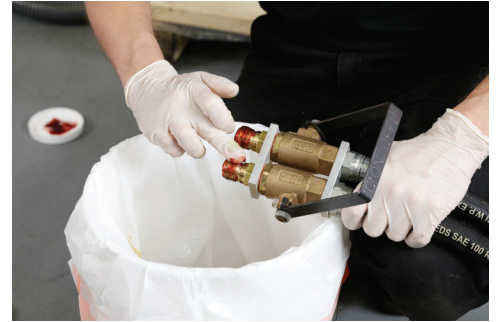
15) Apply a coat of grease to the quick connects on the manifold handle.
