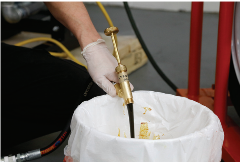
19) Run two cycles of product through the system into the waste bucket to flush the remnants of the cleaning solution.
