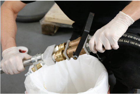
16) Holding the manifold handle in one hand, pull up on the female quick connects. Attach the manifold end to the handle and press down until it locks in place.
