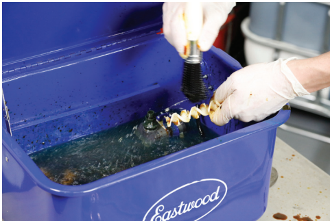
16) Clean mixing elements in the solvent and store them in a safe place to avoid breakage.
