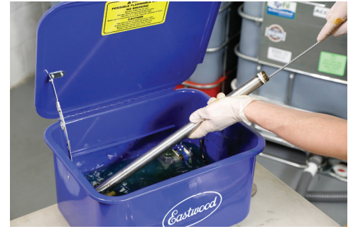
15) Clean the mixing tube with a brush. Place the mixing tube in the solvent.
