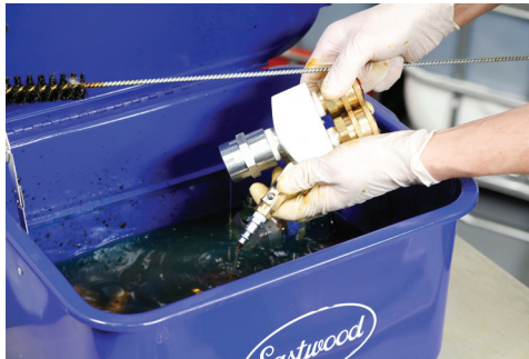
17) Open the manifold head pressure gauge valve and clean the manifold head connectors. Store the manifold head in the solvent.
