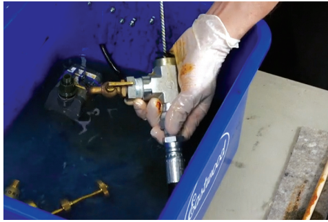
14) Lay the whip hose in solvent and clean the sample drain valve with a brush. Make sure the sample drain valve is open.
