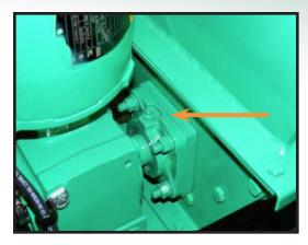
Hopper Auger Bearing Location: Auger gear box
