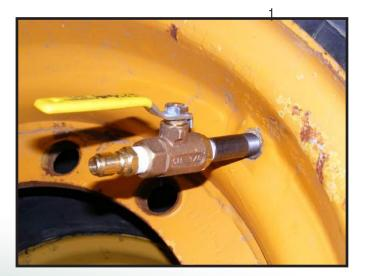
Screw the ball-valve stem adapter into the stem port. Open and close the ball-valve handle to check for proper clearance.
