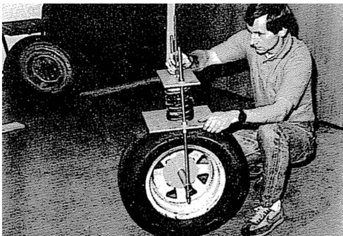
Fig. 23 – Yoke and automotive spring fixture is tightened to impose curb weight of vehicle on which it will be road tested
