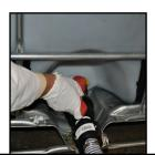
8. Pump 5 strokes into scrap container. Take cup sample from haltec valve.
