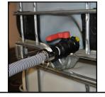
6. Turn on main air valve. Set main air regulator to 90 psi.
