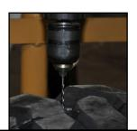
17. Remove safe-fill needle, insert screw into vent hole.
