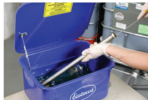
15) Clean the mixing tube with a brush. Place the mixing tube in the solvent.
