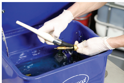
13) Clean the fluid gun plunger in solvent.
