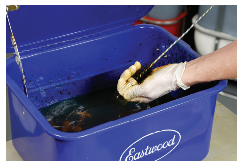
18) Clean the gun stem connector and store in solvent.
