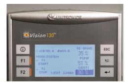
12) Change the cavity speed to 30% then press the enter key. For the F1 and F2 keys on the main control panel to function, the remote switch must be in the "System" Position.
