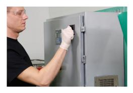
4) Turn the power switch on the control panel to the ON position.
