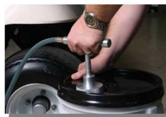
Fig. 3 – Pull up on the handle and inject the proper amount of ReSeal into the tire. Each stroke delivers 6 ounces.
