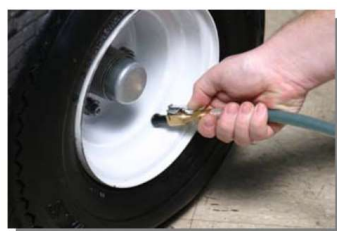
Fig. 2 – Attach the brass connector from the ReSeal pump to the valve stem.
