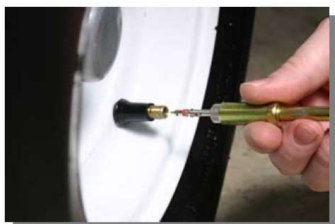
Fig. 1 – Position the valve stem between the 4 and 8 o'clock position and remove the valve stem. The tire will deflate.
