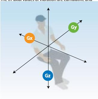
will be amplified to the driver. WBV is now being explored using these measurements to provide meaning to driver fatigue, discomfort, and injury. All three are happening simultaneously and can be observed in the driver.
