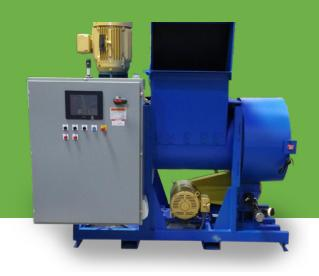
The TyrFil patented AutoFil-GenII can mix virgin tire fill with rubber crumb, PU grind or both rubber crumb/PU grind. The TyrFil Recycling Technology's
