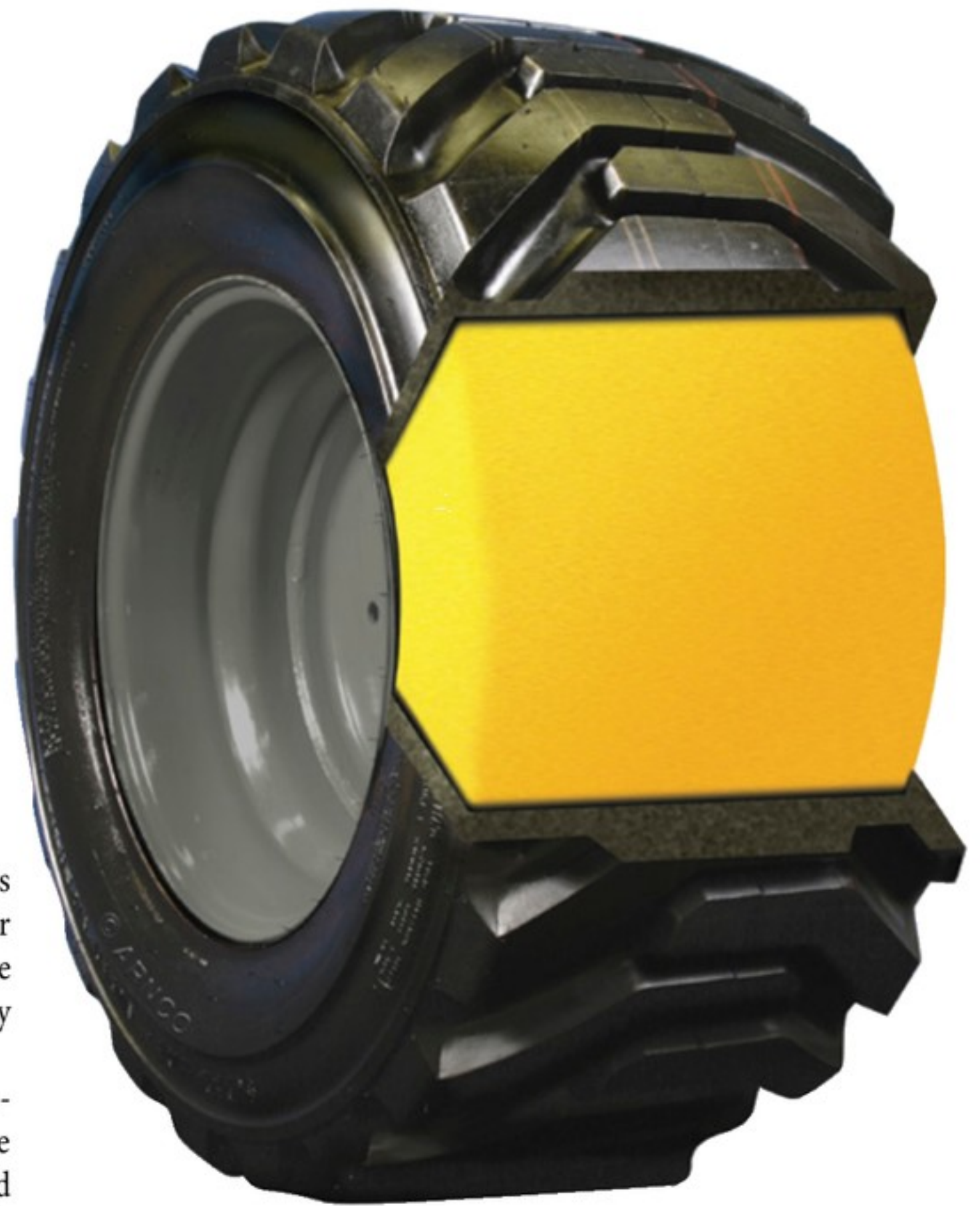
In a filled tire, semi-solid polymer replaces the tire's air.
