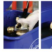
11) Thoroughly clean the gun body and stem connector, rinse and store all parts in alcohol.
