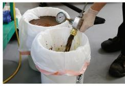
5) Press the jog button on the remote and run half the solvent into the waste pail.
