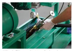
7) Place the fill hose over the mixing well and press the jog button. Allow material to circulate for 30 seconds through the system.
