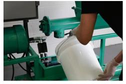
4) Pour the pail of solvent into the mixing well (approximately 2 and a half to 3 gallons)
