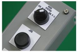
1) After the last tire has been filled and you are ready to shut down the GM, change the mode select switch to "JOG" P.C. on the system remote.
