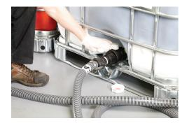
12) Shut off both tote valves and turn off at the main power source.
