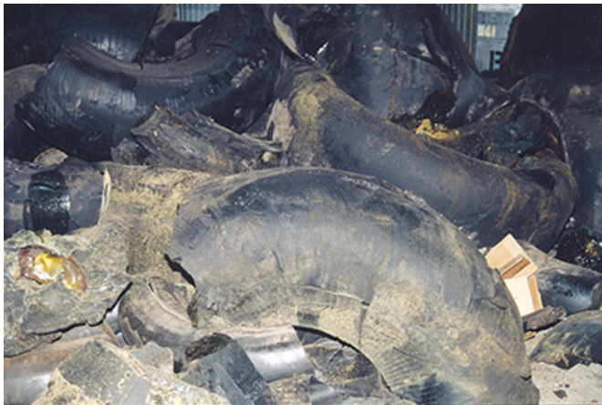
Photo III: This photo shows the wide diversity of old fill used as chunking material in new tires. Many of these pieces were chunk of chunk of chunk.
