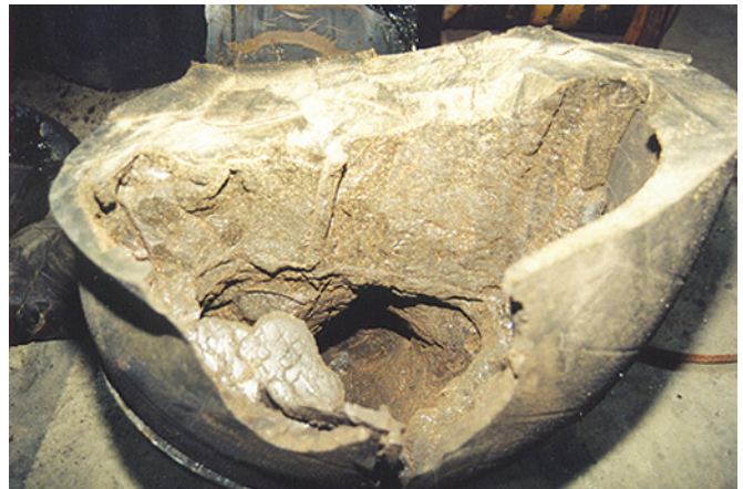
Photo IV: This picture shows what happens to a tire when the “Chunk” overheats. The “Chunked” core has disintegrated while the new virgin fill remained intact encapsulating the “Chunk”. The tire failed due to the failure of the chunk – it had approximately 2” of good tread life remaining when the carcass failed.
