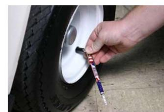
Fig. 4 – Inflate tire and check for proper operating pressure.
