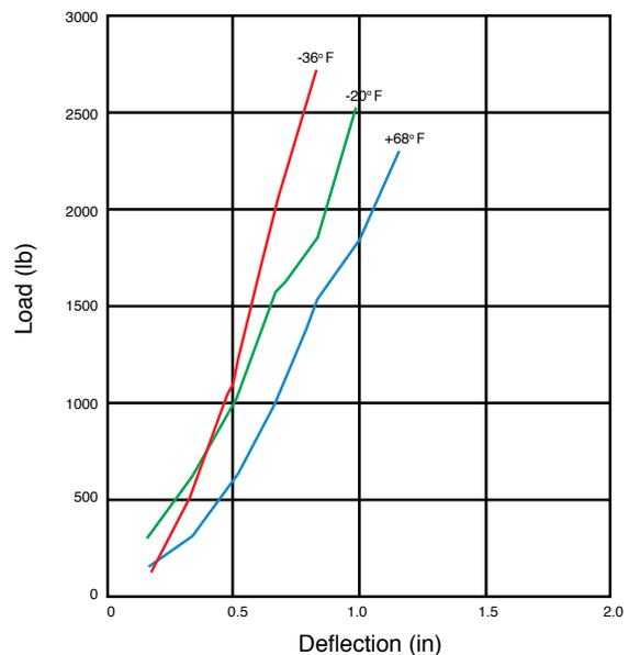
Fig. 22- Load-deflection curves of RePneu filled tire at several temperatures produced on above MTS equipment
