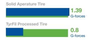
TyrFil Processed Tires – 41% less G-force transmission to cab/operator than solid aperture tires. Data was collected on a front-end loader tested on a track replicating real jobsite conditions.
